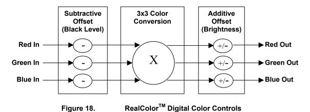
This structure can accommodate all RGB color controls such as black-level (subtractive stage), contrast (multiplicative stage), and brightness (signed additive offset). In addition, it supports all YUV color controls including brightness (additive factor applied to Y), contrast (multiplicative factor applied to Y), hue (rotation of U and V through an angle) and saturation (multiplicative factor applied to both Y and V).
