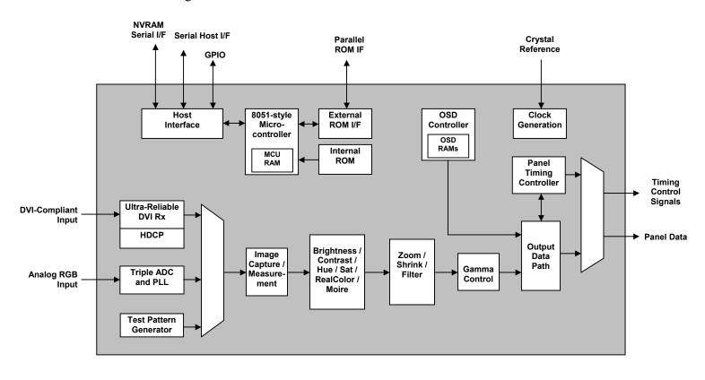
Figure 3. gm5115/25 Functional Block Diagram
