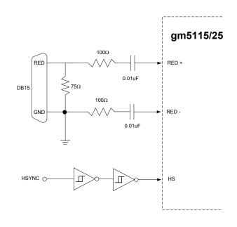
Figure 10. Example ADC Signal Terminations
