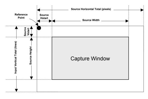
Figure 12. ADC Capture Window
