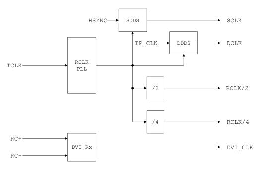
Figure 8. Internally Synthesized Clocks
